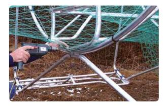
**16.** Lock the inner netting to the upper part of the box holder hatch by using the flat iron.
