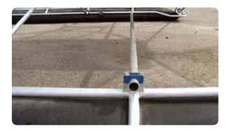
**11.** Attach the hoses to the hose connections of the pontoons. Use the hose clamps. Make sure to leave a bend on the hose to avoid wrinkles/folds.
