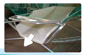
Push the box down (sit inside it) so that the inner netting is locked in between the box and box holder. Drill holes through the box holder by drilling through the pre-drilled holes of the box.
