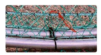
**26.** Use the bottom and top ropes from the adapter to tie the two rings together. The adapter netting should be in between the rings.
