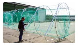
8. Attach the pontoon holders to the benders on the fish chamber. Place the pontoon holders so that the bent end of the pontoons is placed backwards (towards the adapter+wings).
