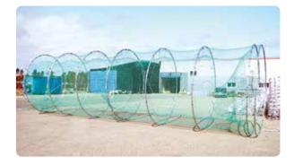
3. Twist the chamber and attach the long aluminium tube with 4 plastic clamps with screws M8x45 mm and bricks on the inside of the top centre of the first 4 rings.
